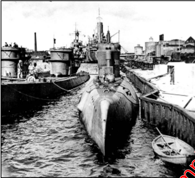
U-3008, a German Type XXI submarine, at Wilhelmshaven, Germany, in June 1945. The two Type IX submarines with her are U-806 (far left) and U-155.
